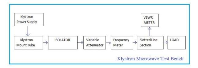
The figure-1 depicts klystron microwave test bench. It consists of klystron power supply, klystron mount tube, isolator, variable attenuator, frequency meter, slotted line section, VSWR meter and load. Let us understand functions of each in brief.
